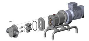
• Remove the lobe screws (25) using a wrench that can see on the following figure and it could deliver by Inoxpa. These screws are threaded to the right. Wooden or nylon blocks can be placed between the lobes to stop them from rotation (blocks position: one to the left in front of the top lobe screw and the other to the right in front of the lower lobe screw).
